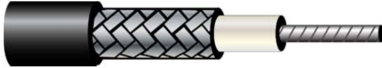
Fig 11. Structure of Coaxial Cable
